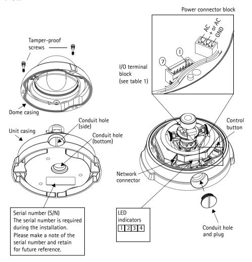
**Power connector block** - for connection of a power supply. See *Power connections*, on page 50.
